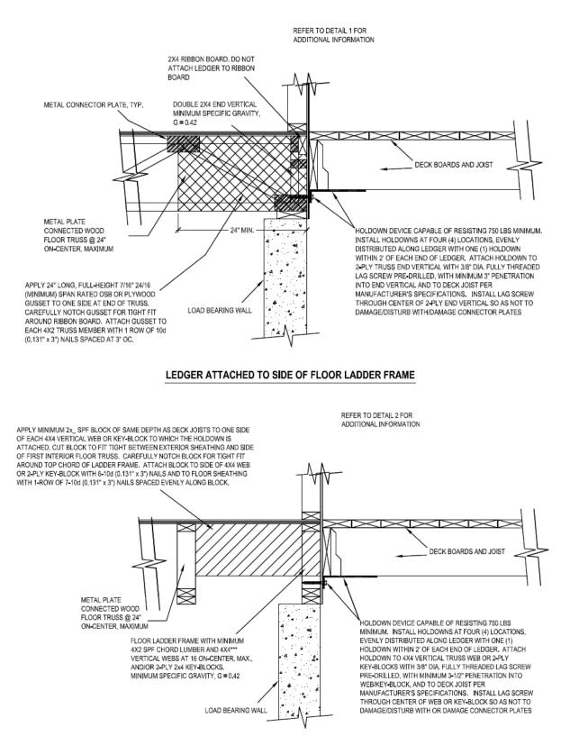
Detail 3: Deck Lateral Load Connection Capable of Resisting the 1500 lbf Lateral Load Requirement Specified in 2009 & 2012 IRC Section 507
