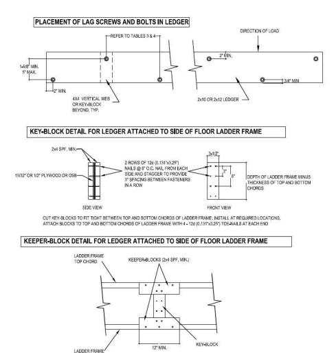
Detail 2: Attachment of Deck Ledger to Floor System with MPCW Trusses,
