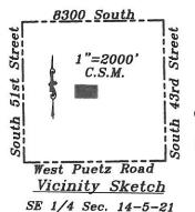
Map bearings refer to Grid North of the Wisconsin State Plane Co-ordinate System, South Zone, with the West line of the SE 1/4 of Section 14, T5N, R21E having an assumed bearing of N 00°08'26" W.
