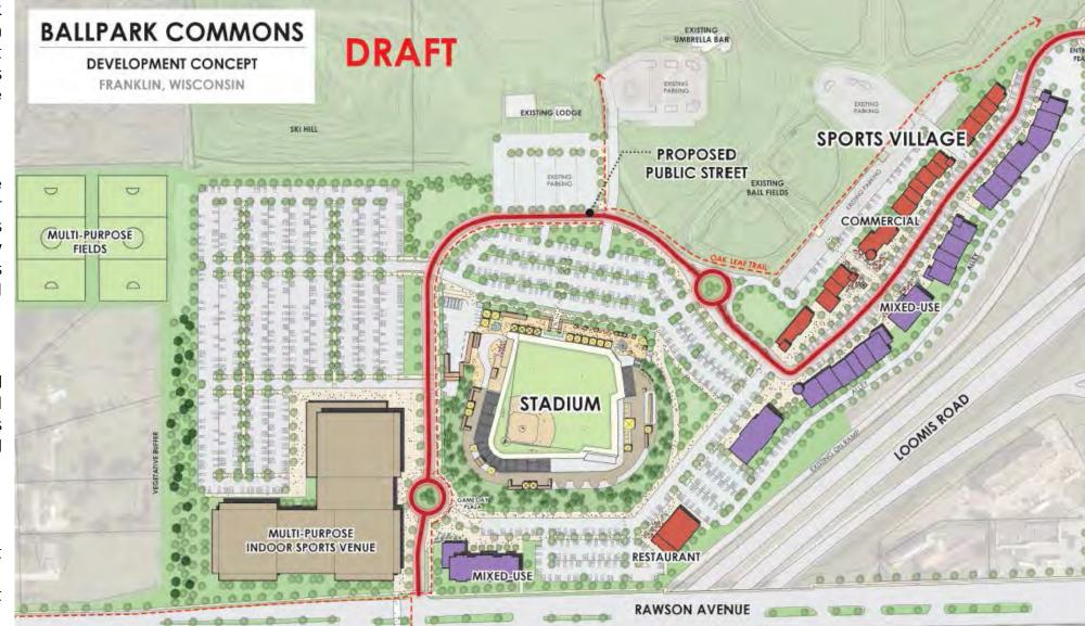
The public street identified in red above shall be constructed to City of Franklin standards including a minimum 40' curb to curb with privately maintained parkways and sidewalks on each side. According to the plan as presented, we also anticipate creating substantial on-street parking to support the mixed-use and commercial uses along the street. This may result in a larger ROW cross-section. We anticipate working collaborative with the City to arrive at the appropriate solution.
